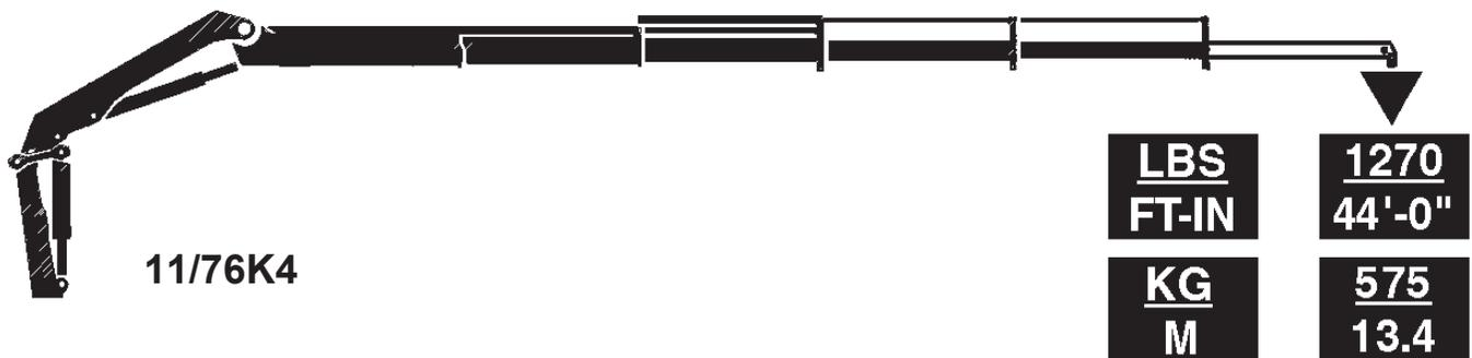
The load capacity limits shown above must never be exceeded.
