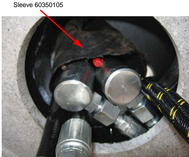
Viewed looking up from crane box. The pressure, return, and rotation hoses are wrapped in the 60350105 hose sleeve.
