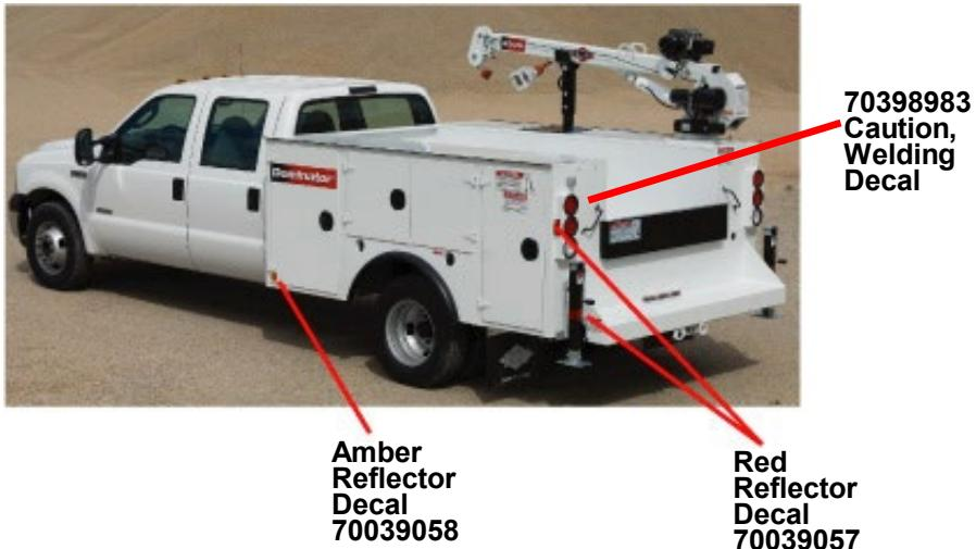
Four red reflector decals, 70039057, are located on each side and outer edge of the tailgate as shown.
