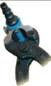
**NOTE:** Stepless ear clamps can only be used once. When removed, they must be discarded and replaced with new clamps.
