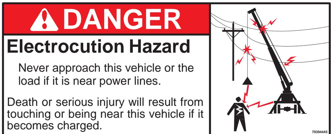
**DECAL:** Electrocutation Hazard-Remote Control Operation
