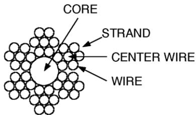
The greatest difference in wire ropes are found in the strands, which may vary widely in the pattern and number of wires laid together.
